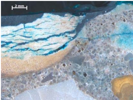
Cross sectional view of a CDP-caused popout
